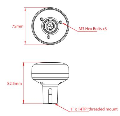
The GPS150 is supplied with 10m of cable and this should be routed through the vessel to a suitable dry internal location where it can be connected to the boat's DC power system and the equipment it will be interfaced with. The cable can be shortened, lengthened or joined without problems.
