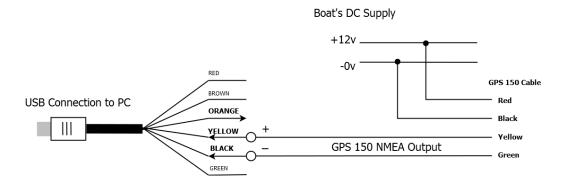
The GPS150 can also be used wirelessly to send GPS data to an iPad/iPhone or Android device by using one of Digital Yacht's WLN10 (4800 baud) or WLN10HS (38400 baud) Wireless NMEA Servers. The GPS150 should be connected to the WLN10/WLN10HS as shown in the diagram below.
